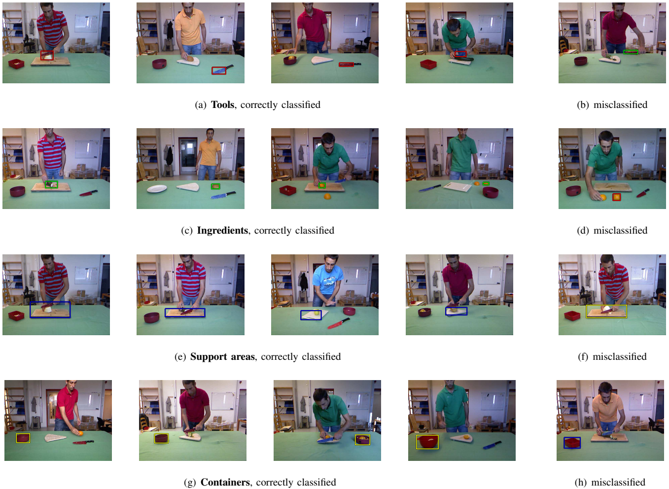
Fig. 9. Examples of classification results using the functional features. Bounding box color coding: ● = Tools, ● = Ingredients, ● = Support areas, ● = Containers.
